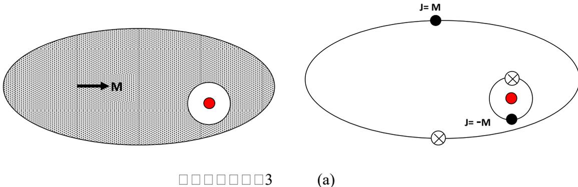
(b) A magnetised ellipsoid with one atom isolated
