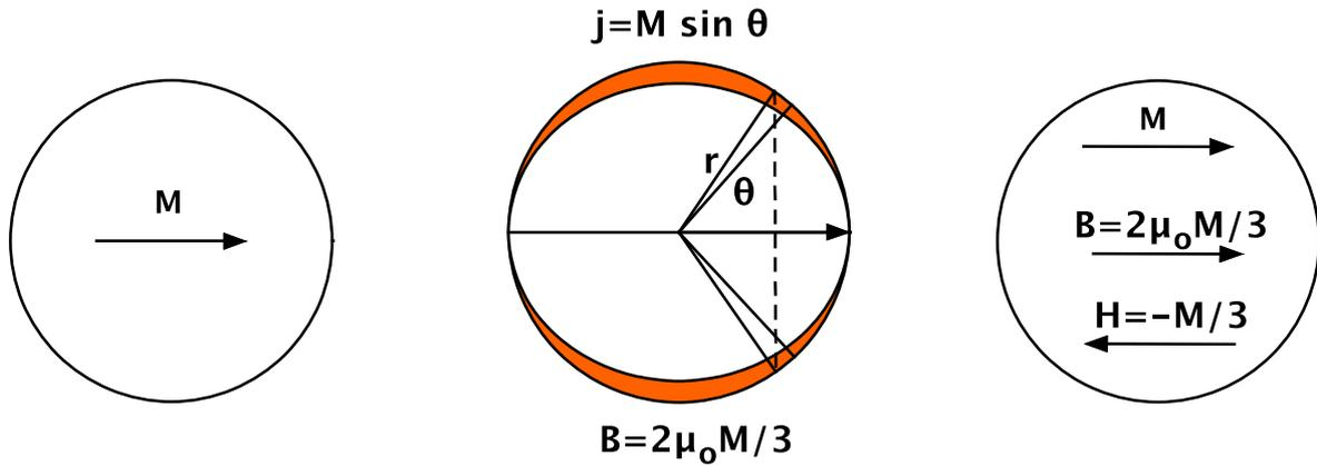
Fig.3a. A Uniformly Magnetised. Sphere
