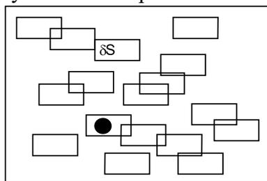
Fig.2. A random array of dipoles in a thickness  $\delta l$  projected onto the  $xy$  plane. The dot is the projection of the line element  $\delta l$  perpendicular to the paper. It happens to intersect a current in this plane
